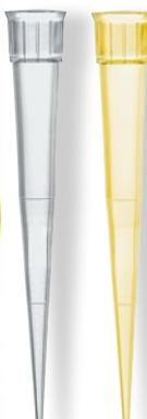
PP, non-sterile with graduation at 20 and 100 µl. Length: 50 mm. Tip-Box with yellow mounting plate for easy identification; palletized tips are colourless. Tips in bags are coloured yellow.
