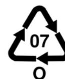
SPI number 07 stands for "other". This is used to indicate other plastics such as PMP, PFA, PTFE etc. VITLAB doesn't use the "0"; rather, it identifies the specific raw material with the abbreviation according to DIN 7728 to simplify identification of the plastic for the end user.
